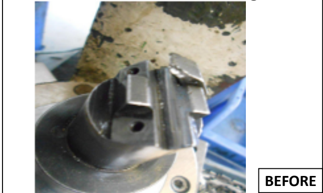
Roll of D shape provided in the roller to avoid the wrong insertion of roller in fixture during pin pressing
